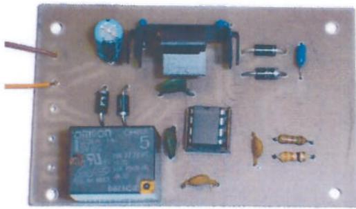
**Figure 11** — Assembled upconverter board — ready for final assembly.
