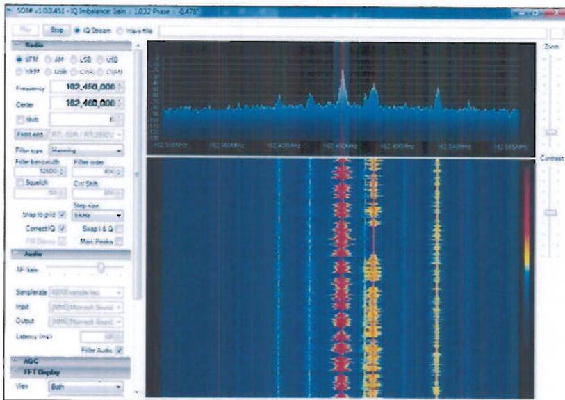
Figure 6 — SDR# Installed screen showing broadcast FM spectrum.
