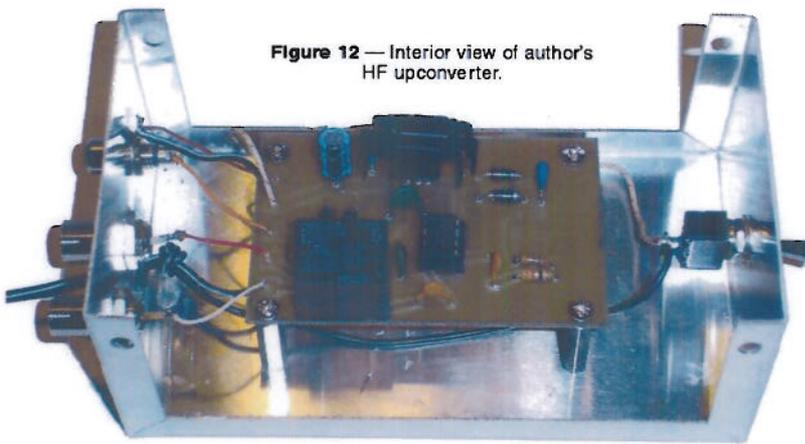
**Figure 12** — Interior view of author's HF upconverter.
