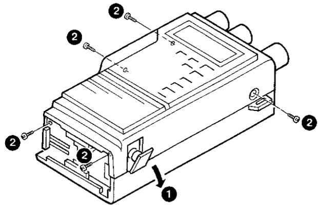
3. Remove the front case from the panel side (3). The panel is firmly engaged with the front case.
