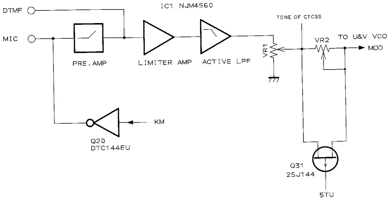
Fig. 3 Modulation circuit
