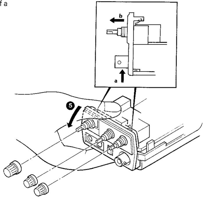
6. To place the IF unit on its side, disconnect the IF signal line connector on the UHF side (6).
