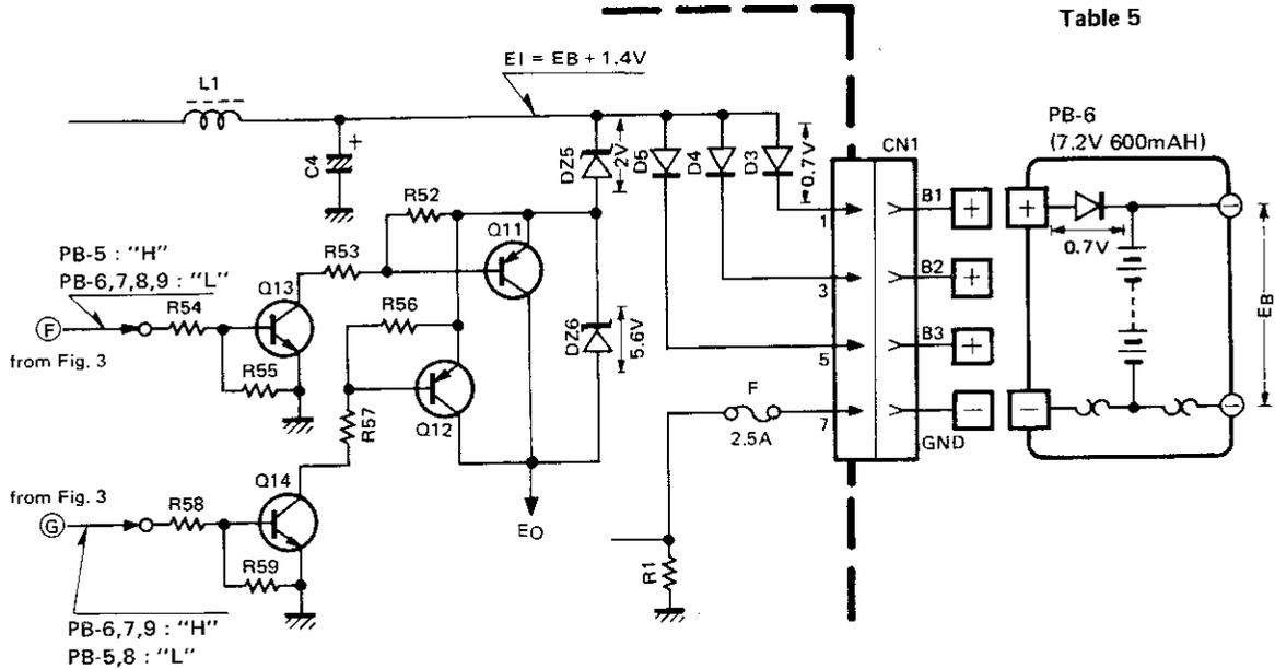
Fig. 5 Sensor Level Switching Circuit Block Diagram
