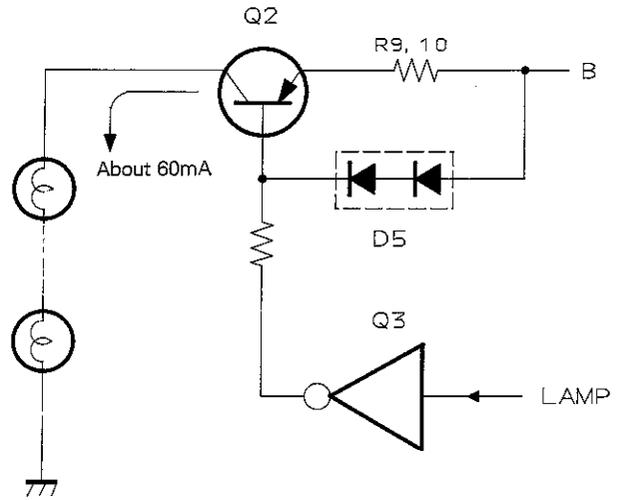
Fig. 10 Lamp circuit
