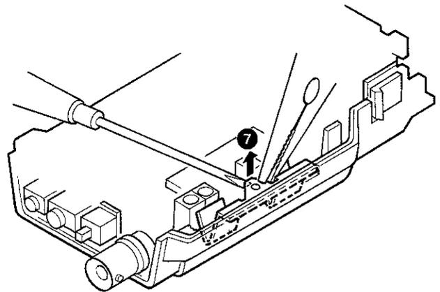
9. To place the TX-RX unit on its side, use a screwdriver from the position shown in the figure; never hold the SP jack, HI/LO switch, or BNC receptacle (9).
