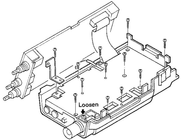
8. Removing the helical plate spring (7)
