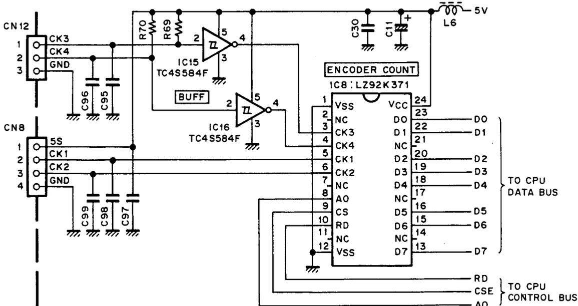
Fig. 26 Encoder circuit
