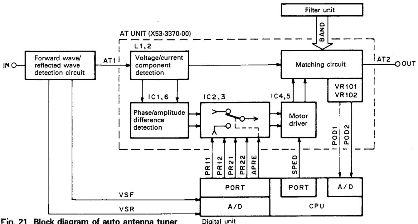
Fig. 21 Block diagram of auto antenna tuner
