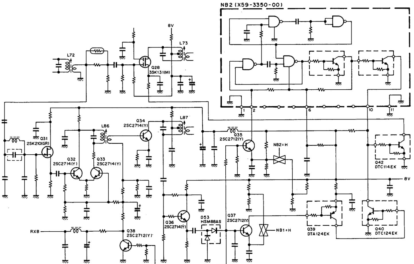
Fig. 8 NB circuit
