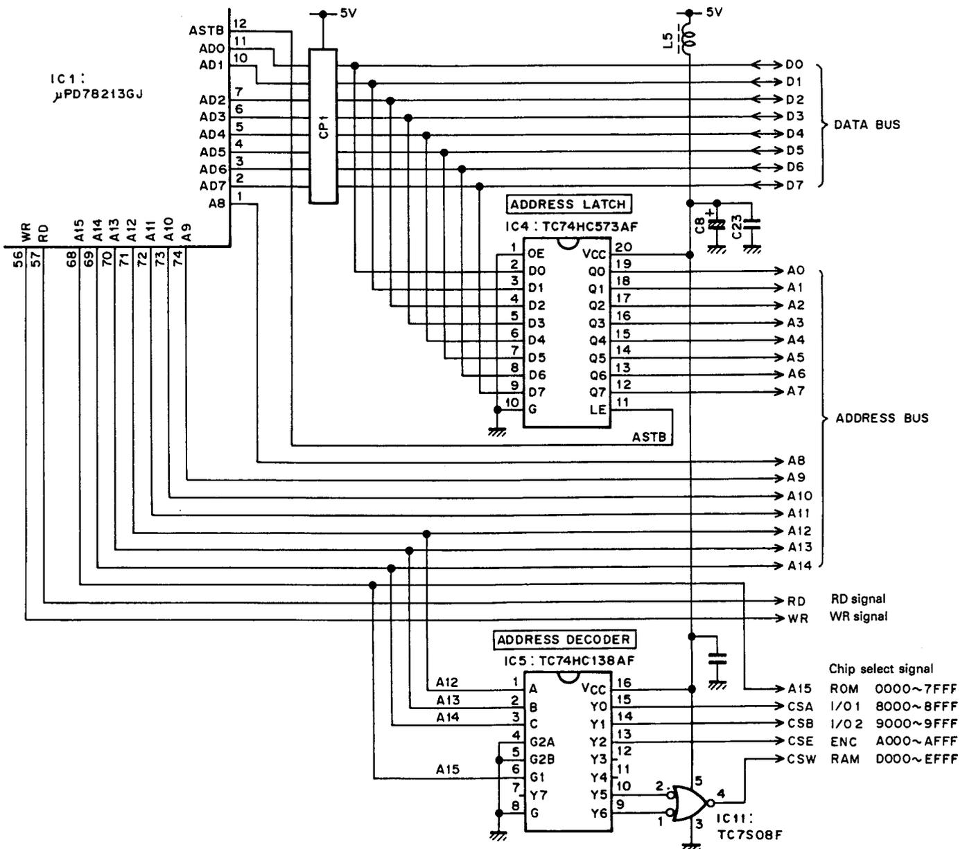
Fig. 23 Address separation circuit
