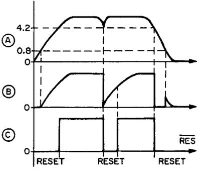
Fig. 25 Reset circuit
