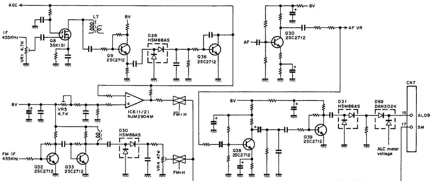
Fig. 12 AGC, signal-strength meter, and dB meter circuits
