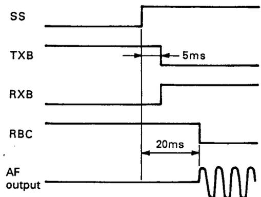
Fig. 17 PLL, DDS data and transmit/receive timing signal
