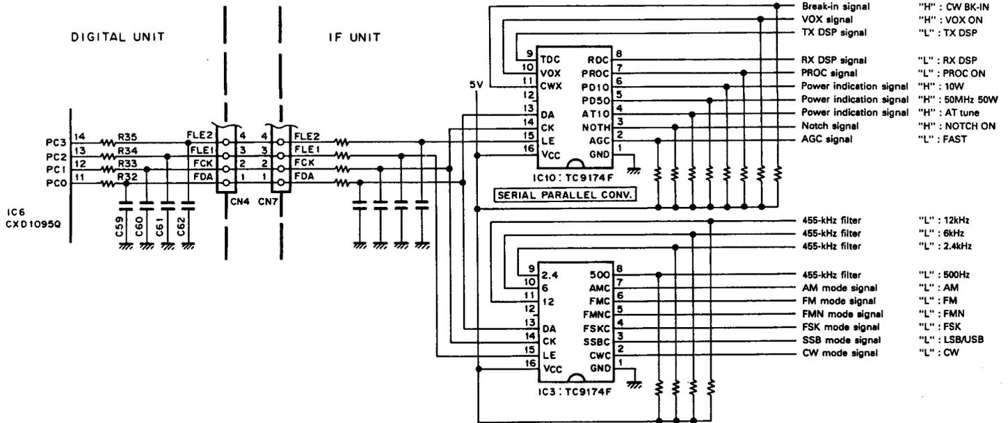
Fig. 27 IF unit serial-to-parallel converter
