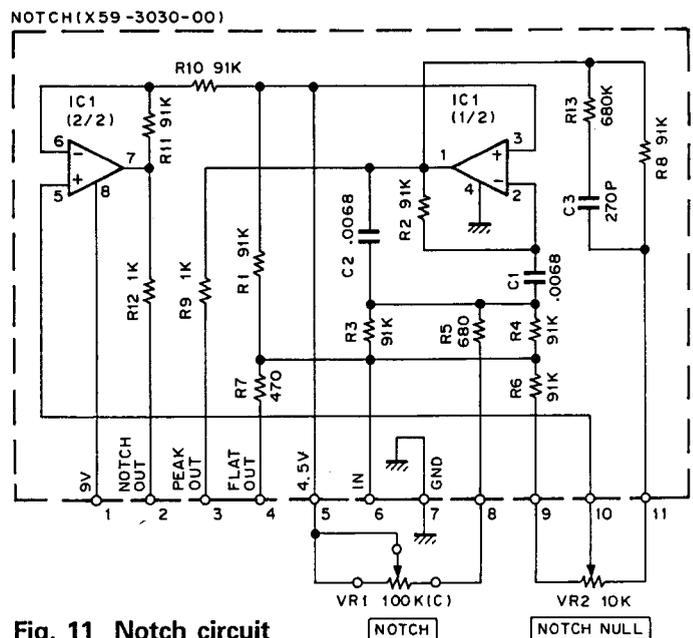
Fig. 11 Notch circuit
