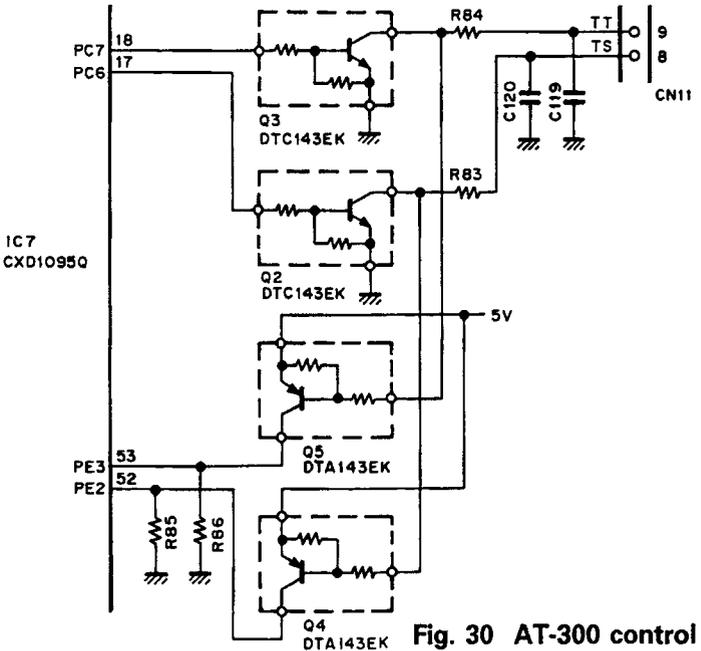
Fig. 30 AT-300 control circuit
