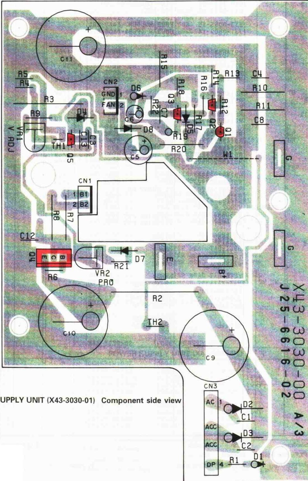
POWER SUPPLY UNIT (X43-3030-01) Component side view
