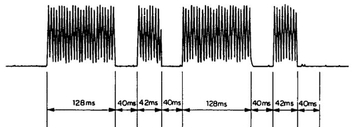
Fig. 33 Output waveform of Morse code C
