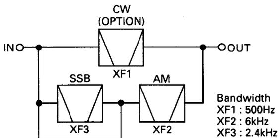
Fig. 7 Filter circuit
