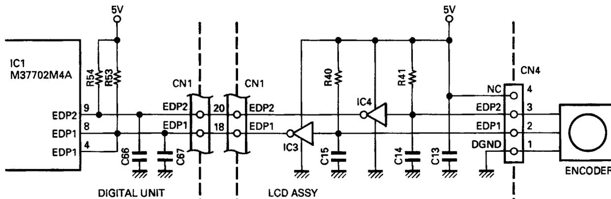
Fig. 18 Encoder circuit
