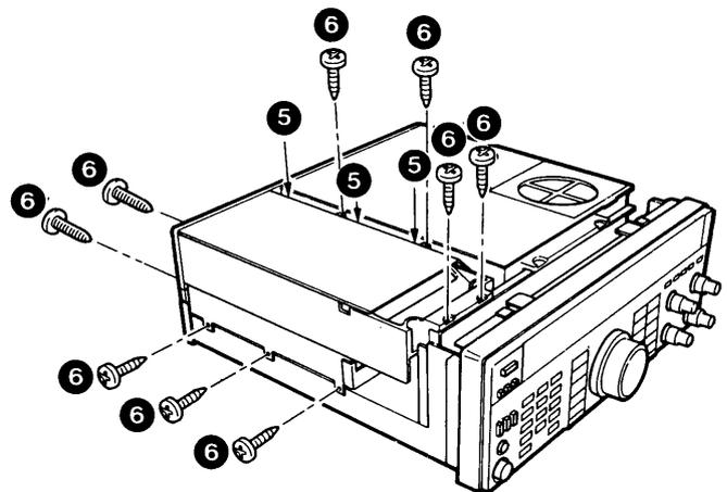
6. Replace the top and bottom covers ( 7 ). Use 5 pan head screws provided with the UT-10 ( 8 ).
