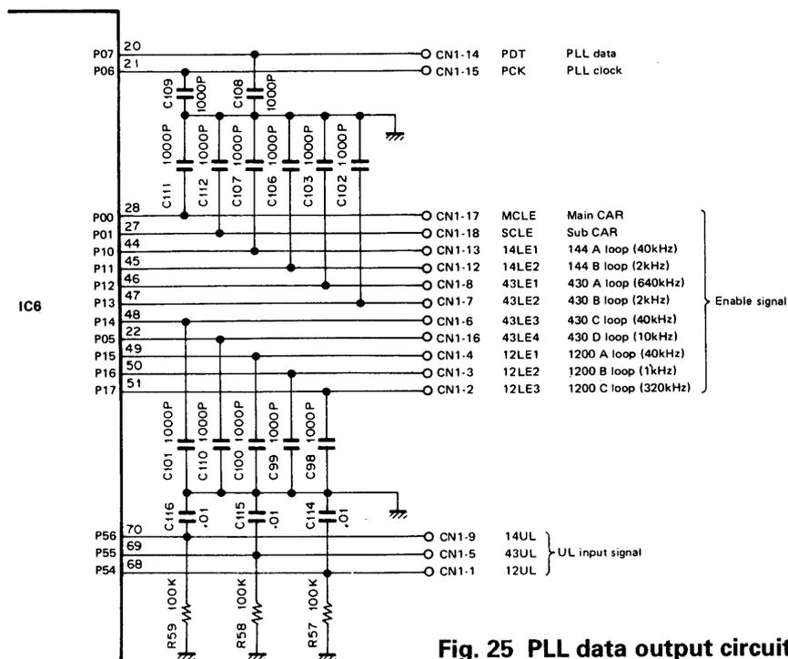
Fig. 25 PLL data output circuit
