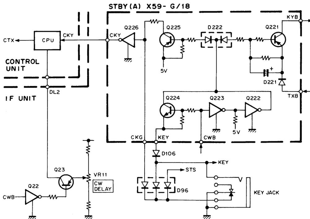
Fig. 9 Keying circuit
