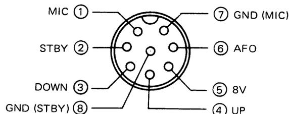
**Fig. 27 MIC terminals (view from front panel side)**
