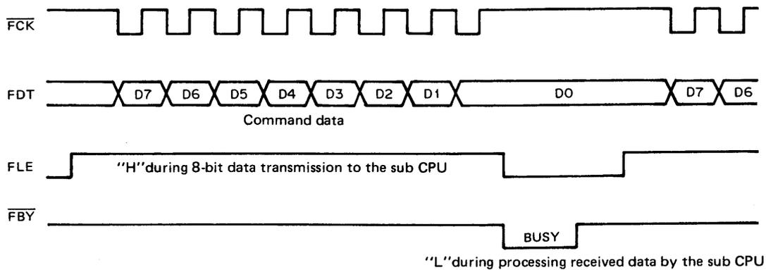
Fig. 24 Timing chart for serial data transmission
