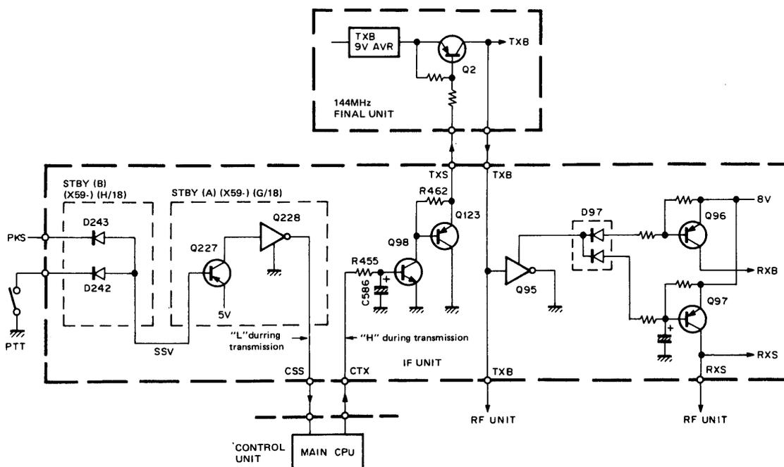
Fig. 8 Standby circuit
