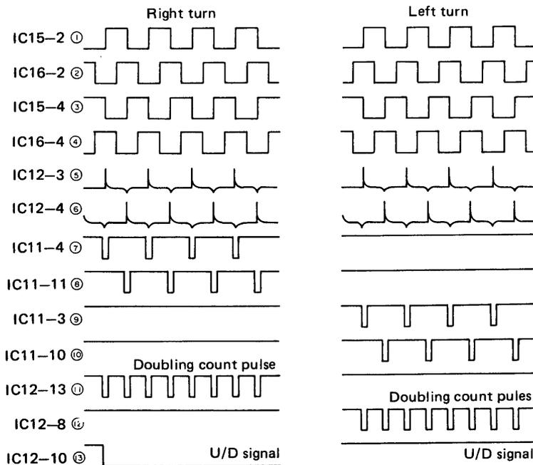
Fig. 19 Timing chart for doubling 250-pulse count signal
